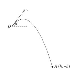
The particle subsequently passes through the point A with coordinates (h, -h) as shown in the diagram. It is given that v = 14 and  $\theta = 30^{\circ}$ .
